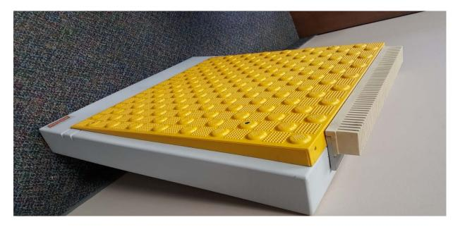
Photo 1 – Sloped precast tactile edge tile with horizontal gap filler for maximum 32 mm vertical gaps.
