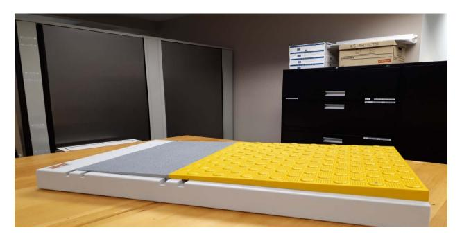
Photo 2 – Sloped precast tactile edge tile for vertical gap corrections in excess of 32 mm.
