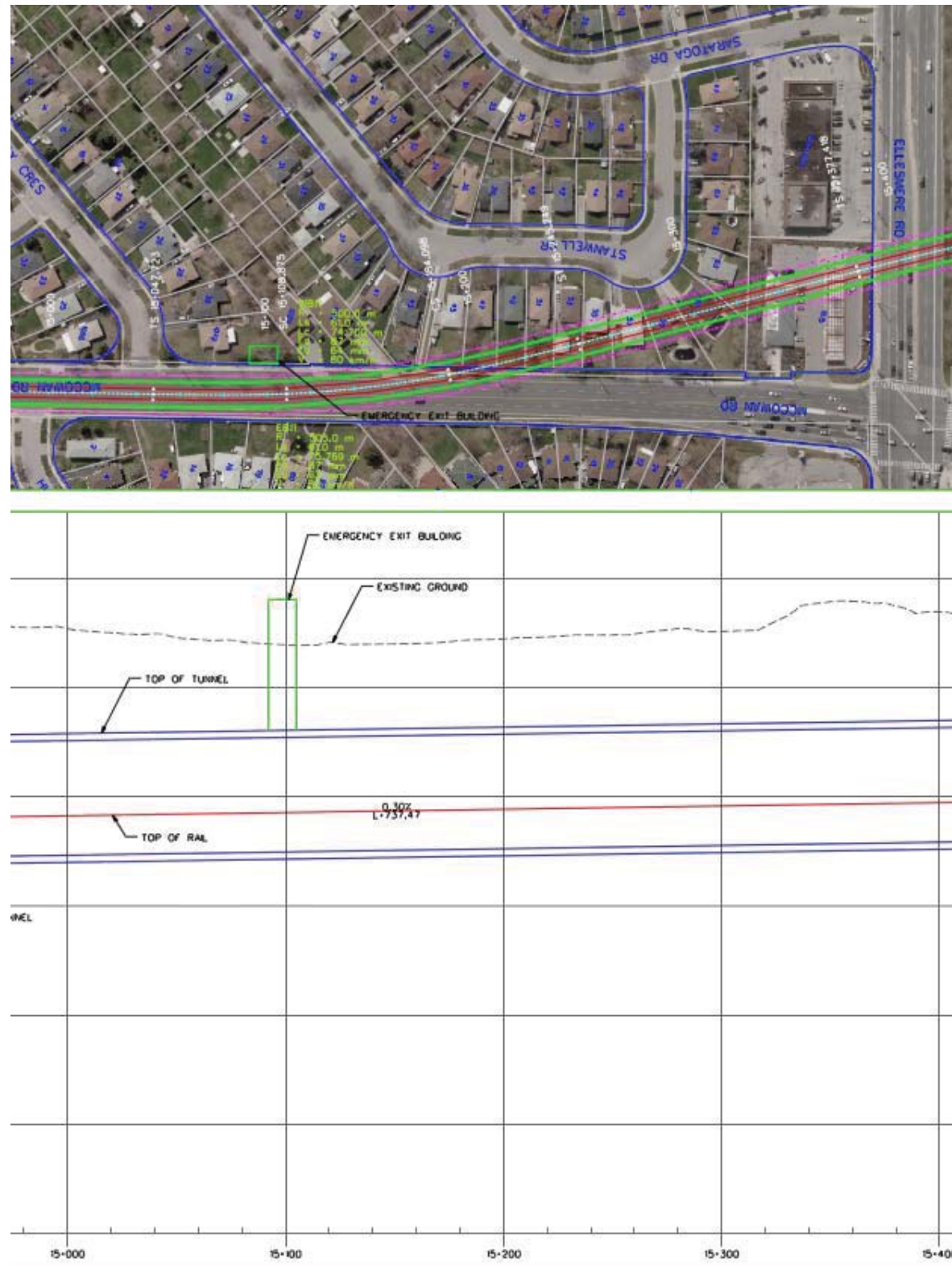
Figure B: Scarborough Subway Alignment and Depth
