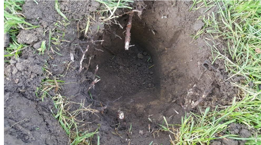
Photo 29: Typical test pit found in the manicured lawn area east of 1360 Danforth Road showing mottling and gravel inclusions; view down
