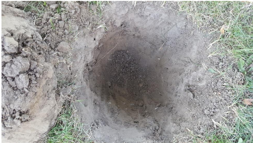
Photo 27: Typical disturbed test pit with soil mottling and gravel inclusions; view down
