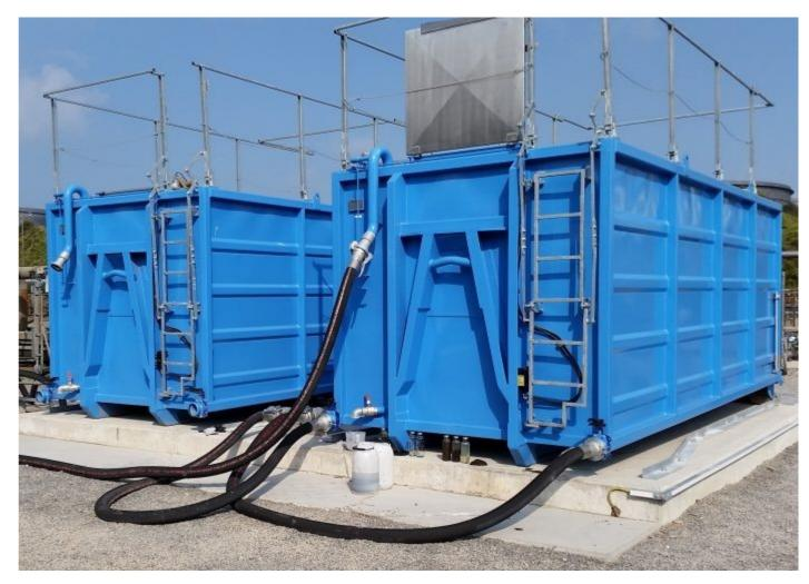
Example of a typical dewatering tank. Tanks used for this project may not look exactly like those pictured.
